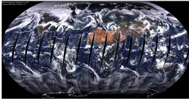
Fig. 3.4: Example of a composite MODIS ‘RGB’ image for a whole day, April 1, 2001. Images are known as ‘RGB’ or ‘True-Color’, created by merging MODIS observations in 0.47, 0.55 and 0.66 \mu\text{m} .
