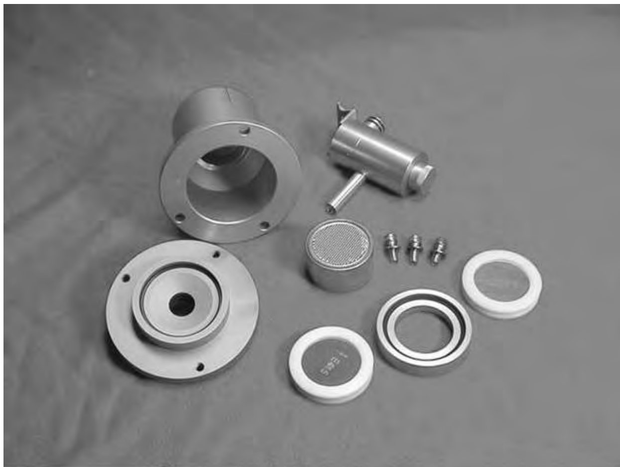
Figure 2-6 Disassembled Met One SASS canister. Courtesy of Met One Instruments, Inc.
