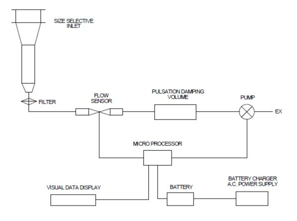
For purposes of this monitoring program, the PQ100 sampler will be operated without the particle size selector and filter holder shown in Figures 5-1 and 5-2. The sampler will be retrofitted with a custom apparatus supplied by ERG. The retrofit replaces the typical BGI F20 filter holder and particle sizing inlet with a section of stainless steel tubing used to attach a Teflon filter holder assembly and glass funnel inlet apparatus.
