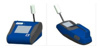
Run **Zero Cal** prior to every 24-hour sampling event. Zero Cal requires that the zero filter be attached prior to running. Zero Cal must also be performed if the unit is reading negative concentrations. It is not possible for the DustTrak monitor to read negative concentrations. Negative concentrations are a symptom of zero drift.
