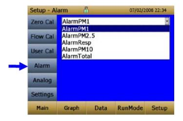
The Alarm is dependent on the logging interval. For the DustTrak to alarm as soon as the Alarm Setpoint is exceeded, the logging interval must be set as low as possible (i.e., 1 second or 2 seconds). If long test durations do not permit setting such a short logging interval, use the STEL alarm instead. The STEL is always based on 1 second concentrations and is independent of the logging interval. For more details on the STEL alarm, see section below on STEL.
