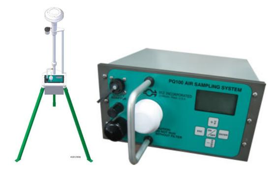
Figure 5-2. BGI PQ100 Sample System
