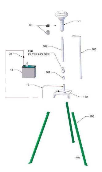
Note: The BGI particle size selector (01), water jar (03), filter holder adapter (161), F20 filter holder, and brace (163) will be omitted and replaced by the retrofit apparatus shown in Figure 5-5.
