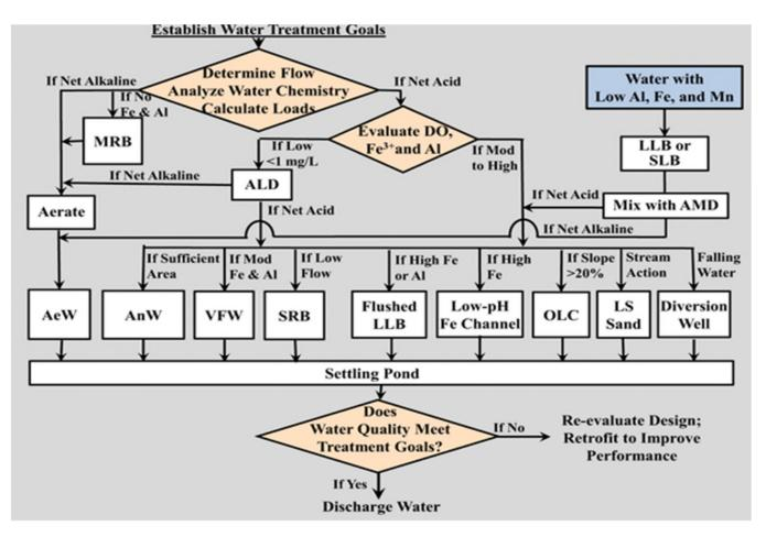
Key: MRB- Manganese Removal Bed, ALD – Anoxic Limestone Drain, AeW – Aerobic Wetland, AnW – Anoxic Wetland, VFW – Vertical Flow Wetland, SRB – Sulfate Reducing Bioreactor, LLB – Limestone Leached, OLC – Open Limestone Channel, LS – Limestone, SLB – Slag Leached
