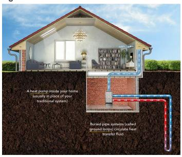
**Figure 1: How Geothermal Works**
