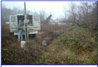
Direct push technology used to collect soil and groundwater samples at the Sauer Dump Site, Baltimore County, MD.
