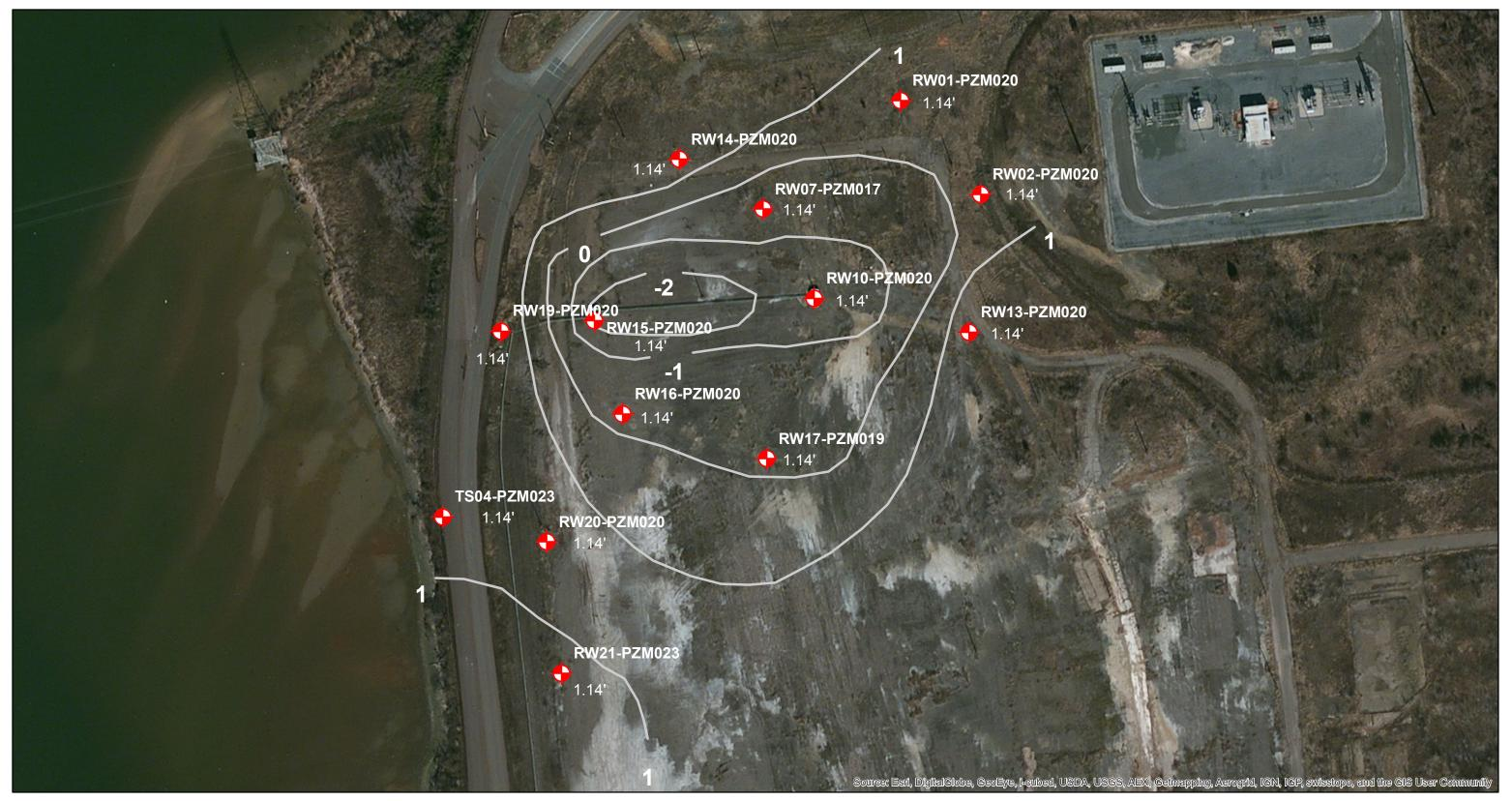
Former Rod & Wire Mill Area Intermediate Zone Groundwater Elevation Contour Map
