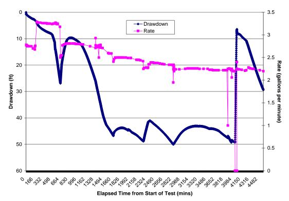
$Figure\ 6-Drawdown\ and\ Rate\ during\ RW-2\ Pumping\ Phase$
