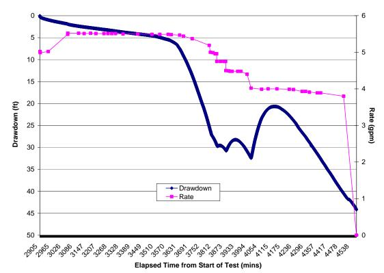
Figure 8 – Drawdown and Rate during RW-3 Pumping Phase
