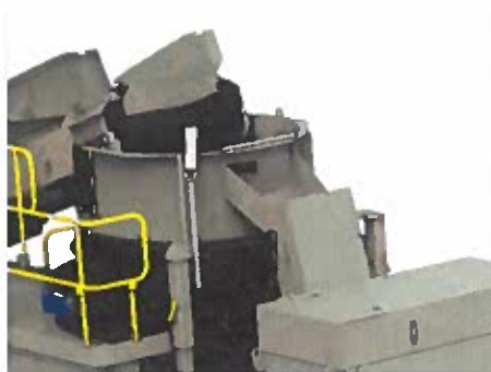
Overflow chute prevents spillage, keeping product moving, and maintaining a clean site.
