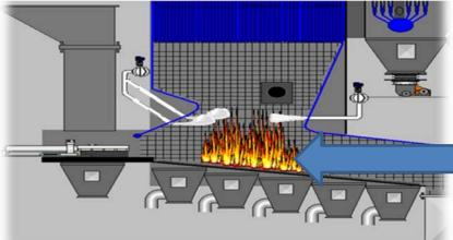
Less intense combustion spread out more in grate zones 2 and 3 (normal) and centered for better temperature distribution in furnace
