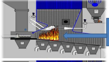
Very narrow intense combustion in grate zones 1 and 2 creating high fuel bed temperature (Higher NOx) and poor temperature distribution in furnace
