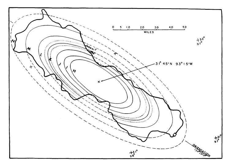
Figure 12. Isohyetal Pattern Placed on Leon River Basin (NVS, 1982)
