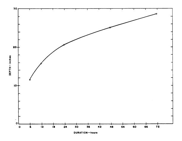
Figure 13. PMP Depth-Duration for 3,000 mi<sup>2</sup> Storm on Leon River Basin
