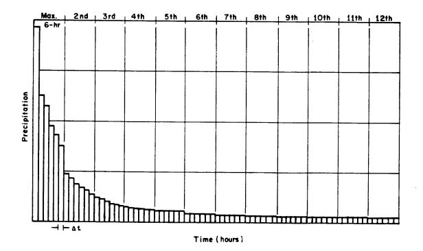
Figure 23. Incremental PMS Depth Histogram
