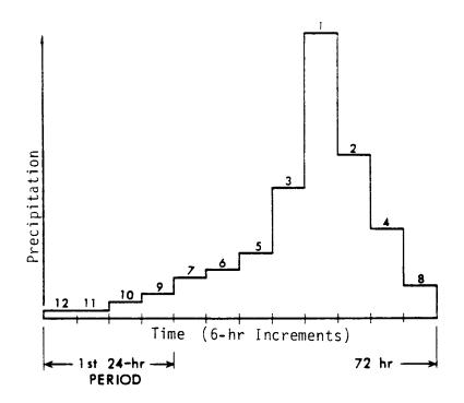
Figure 7. Schematic of One Temporal Sequence Allowed for 6-hr Increments of PMP (NWS, 1982)
