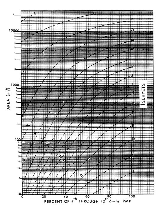
Figure 17. Nonogram for 4<sup>th</sup> through 12th 6-hr PMP Increment (NV5, 1982)
