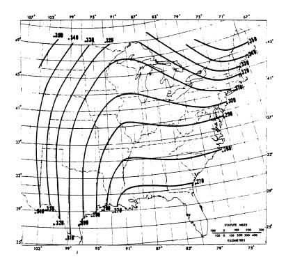
Figure 8. Ratio of 1-hr to 6-hr Precipitation for 'A' Isohyet of a 20,000 mi2 Storms (NVS, 1982)
