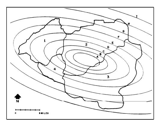
Figure 26. Storm Pattern for Trials 1, 2, and 6
