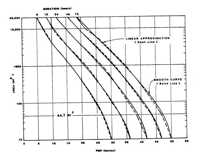
Figure 19. Linear Approximation of Depth-Area-Duration Relations
