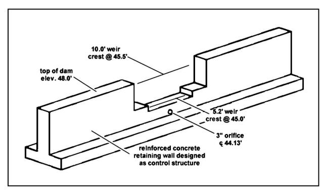
Figure C.1.5 Schematic of Control Structure
