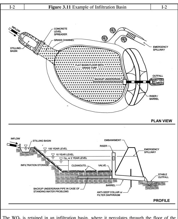
The  $WQ_{\nu}$  is retained in an infiltration basin, where it percolates through the floor of the basin in a two day period.
