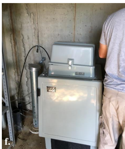
Figures 2a-2f. Pictures from the Moores Run, BACI site visit. (a) instream site, looking downstream; (b) instream site, looking upstream; (c) outfall site, looking downstream; (d) outfall site, looking upstream; (e) instream sampler; (f) refrigerated outfall sampler.
