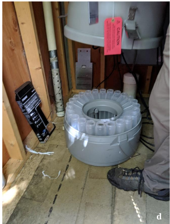
Figures 4a-4d. Pictures from the Airpark Business Center, CACO site visit. Figure a. is the detention pond; b. is the in-stream site with a weir, looking upstream; c. is the outfall from the detention pond; d. is the water sampler.
