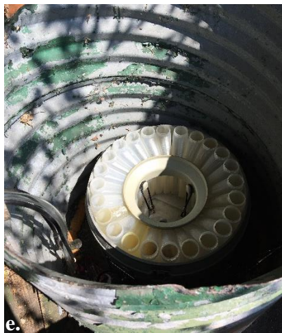
Figures 2a-2f. Pictures from the Moores Run, BACI site visit. (a) instream site, looking downstream; (b) instream site, looking upstream; (c) outfall site, looking downstream; (d) outfall site, looking upstream; (e) instream sampler; (f) refrigerated outfall sampler.
