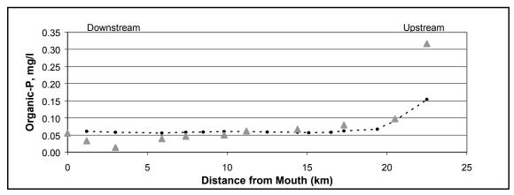
Figure A24: Organic Phosphorus vs. River Mile for the Calibration of the Model (High flow)
