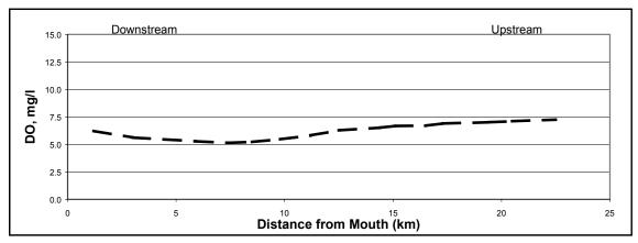
Figure A27: Dissolved Oxygen vs. River Mile for the Baseline Condition Low Flow Scenario
