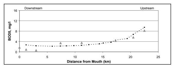
Figure A18: BOD vs. River Mile for the Calibration of the Model (High flow)
