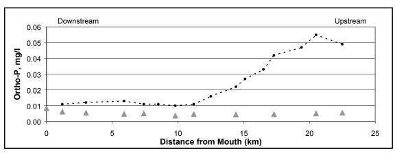
Figure A25: Ortho-Phosphate vs. River Mile for the Calibration of the Model (High flow)
