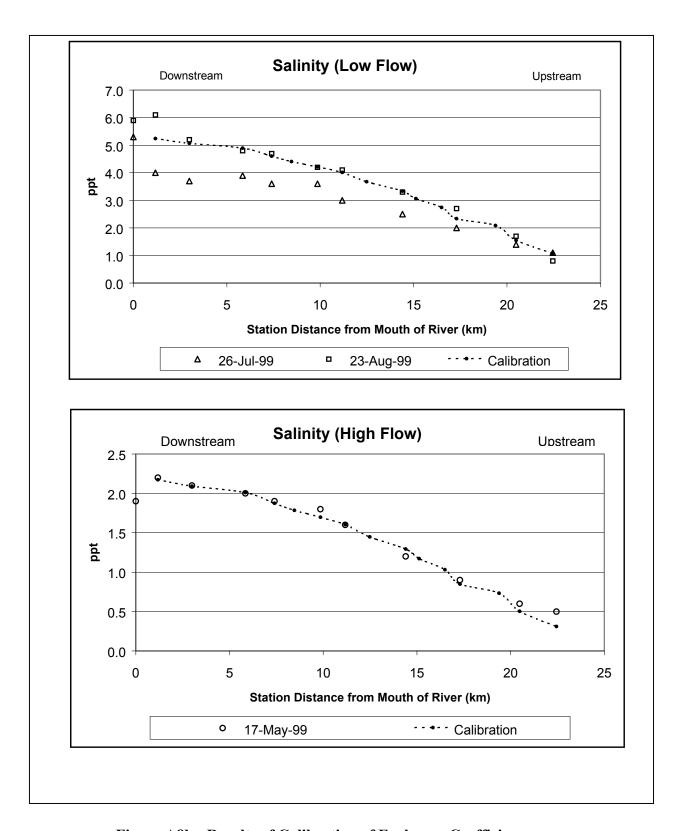
Figure A8b: Results of Calibration of Exchange Coefficiens
