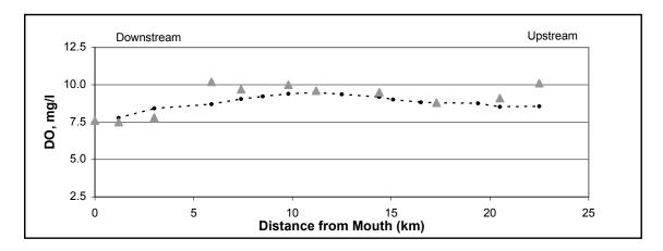
Figure A19: Dissolved Oxygen vs. River Mile for the Calibration of the Model (High Flow)
