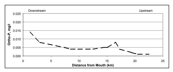
Figure A41: Ortho-Phosphorus vs. River Mile for the Baseline Condition Average Flow Scenario
