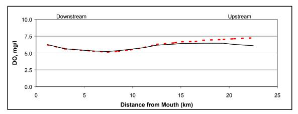
Figure A43: Dissolved Oxygen vs. River Mile for the Future Low Flow TMDL Scenario
