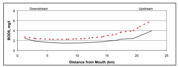
Figure A42: BOD vs. River Mile for the Future Low flow TMDL scenario
