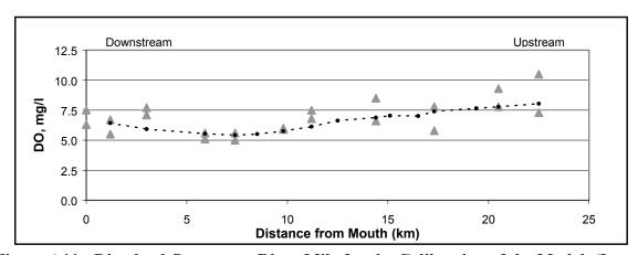
Figure A11: Dissolved Oxygen vs. River Mile for the Calibration of the Model (Low flow)
