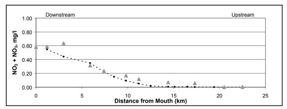
Figure A21: Nitrate (plus Nitrite) vs. River Mile for the Calibration of the Model (High flow)
