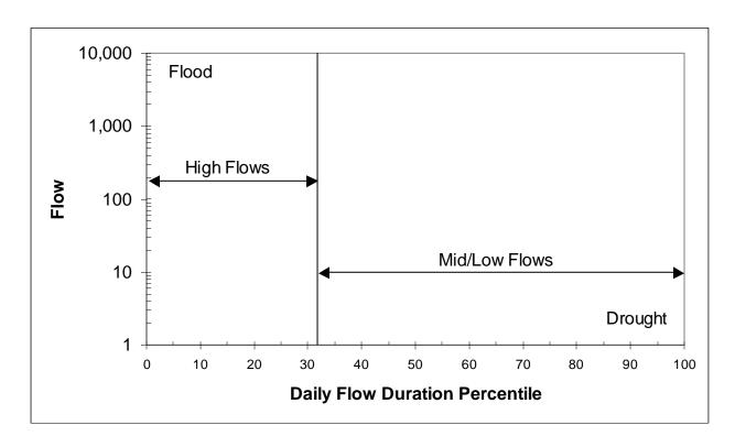
Figure 2.3.1: Conceptual Diagram of Flow Duration Zones
