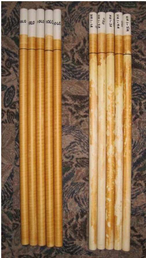
Figure 4. IRIS Tubes on left have not yet been installed, paint is still intact. IRIS tubes on right were in the soil of the wetland mitigation site for four weeks and now show significant paint removed, suggesting soil reduction.
