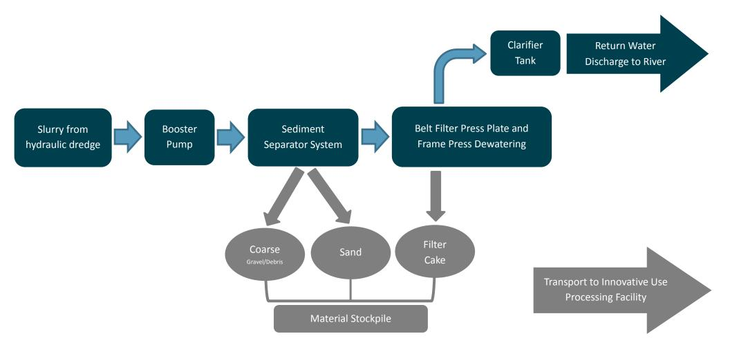
Figure 1. Dewatering process of the dredged material at the staging area
