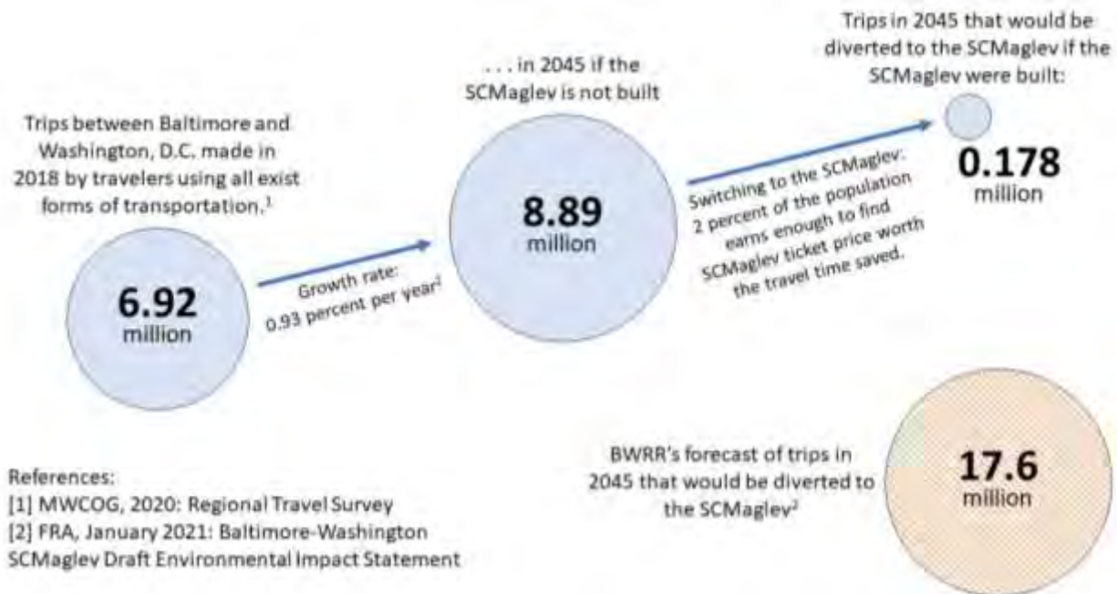
Figure 3. A schematic diagram showing how the present chapter calculates an unofficial forecast for the number of maglev trips in 2045 that would be made by “diverted” travelers. A diverted traveler is someone who would make the trip by another form of transportation if the maglev were not built. The 17.6-million-trip official forecast is much larger than the 178,000-trip unofficial forecast. Both forecasts exclude BWI airport passengers.
