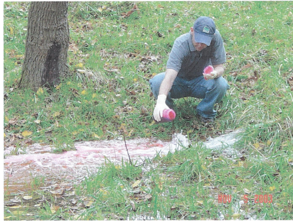
Figure 3. Illustration of Phloxine B inoculation of sinkhole 1
