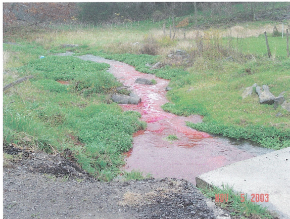
Figure 5. Illustration of rhodamine WT inoculation of Meadow-Brook
