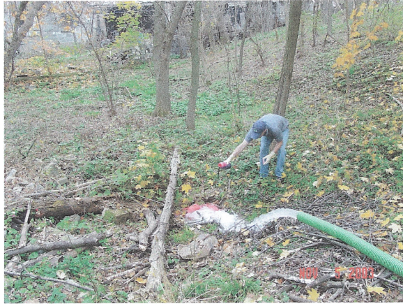
Figure 4. Illustration of Phloxine B inoculation of sinkhole 2
